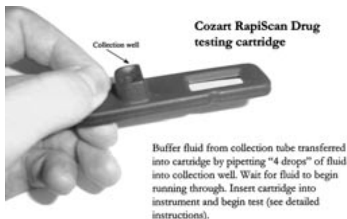
FIG. 1b—The Cozart RapiScan Drug testing cartridge. Buffer fluid from the collection tube is transferred into the cartridge by pipetting “4 drops” of fluid into the collection well.
