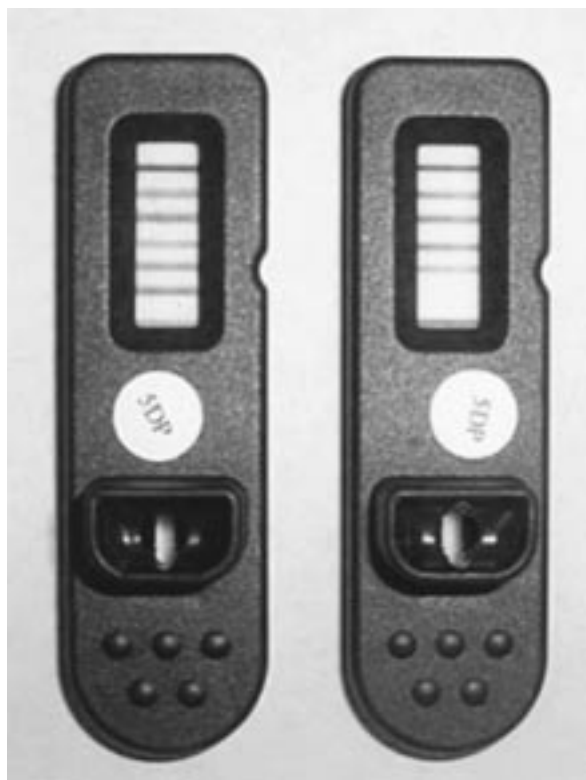
FIG. 1d—the Cozart RapiScan Drug testing cartridge after incubation and test development. The cartridge on the left is negative for all drugs, the cartridge on the right is positive for one of the five drug classes.
